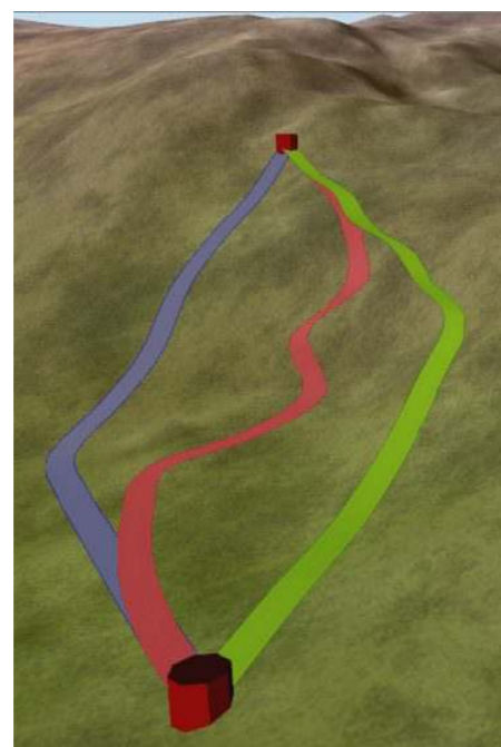
Figure 1 Adaptive roads in Citygen. Blue - Minimum Elevation Red - Least Elevation Diff Green - Even Elevation Diff
